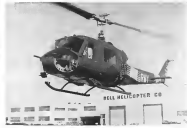
BELL HU-1B WITH 48 2.75-IN. AIRCRAFT ROCKETS
